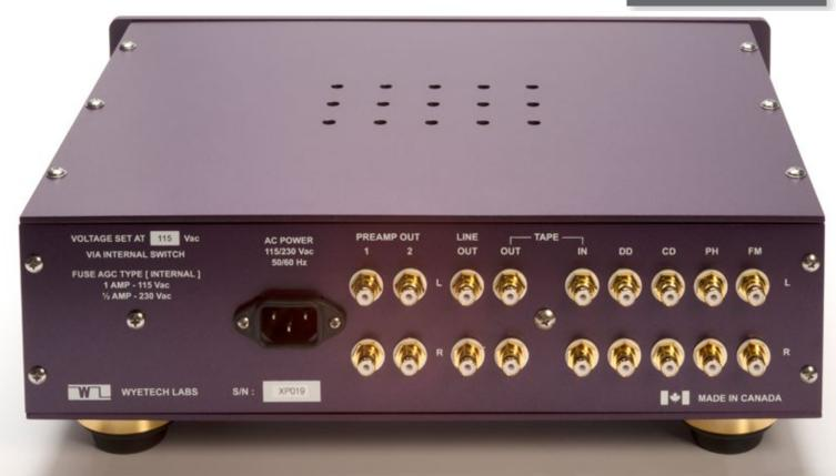
Ruby features only singleended ins and outs. Four source inputs are flanked by the tape loop ins and outs. An additional lineout connection allows a little extra versatility many preamps lack. Rounding out the rear panel are two sets of main outputs. If the owner chooses to send a signal to a subwoofer, for example, Wyetech has you covered.
